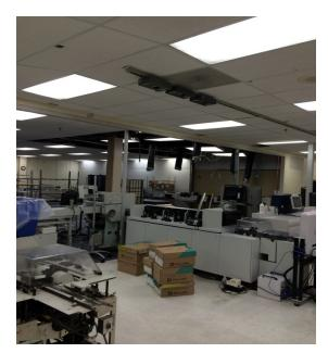
In Phase II, the former postal room will be gutted and converted to VSARA space. This includes new heat pumps, significant electrical and data upgrades, and finishes. New card readers and three door alarms will be added, requiring a new security panel.
