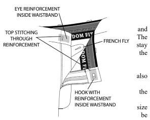
in proportion to waist outlet so seat may also be let out. Seat seam must be sewn with a tandem needle machine (double-needle stitch) for maximum strength.
