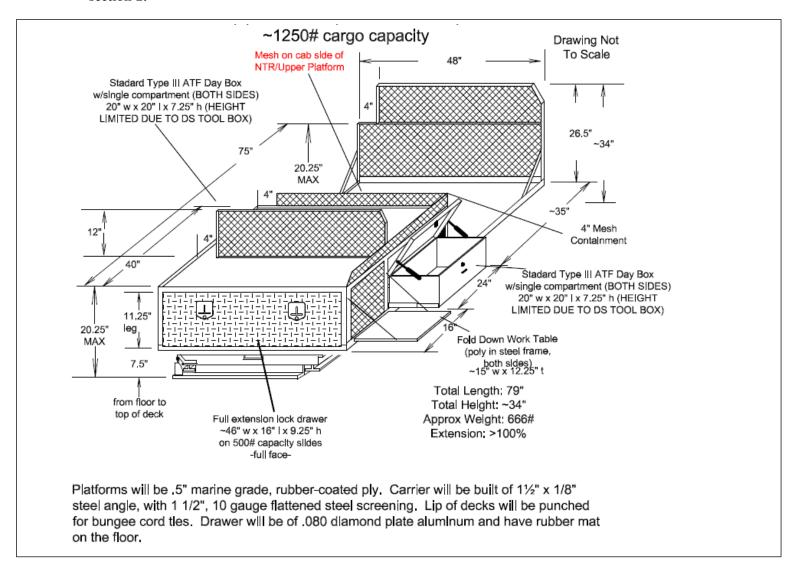
Item 2 – Prop 20539 Adaptable to truck bed lengths of 5.5 Feet, 6.6 Feet or 8 feet as outlined in section 2.
